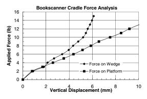
Figure 4. Applied force versus vertical displacement of the spring-loaded platform. The difference between the force applied to the platform alone versus the force applied to the wedge, through the book and to the platform is the additional force directed normal to the book pages
