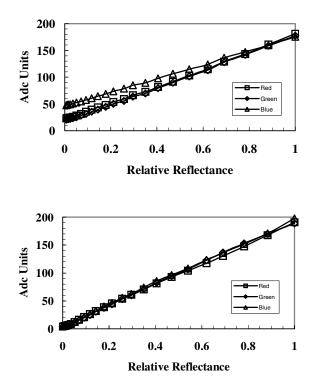
Figure 5. Dynamic range – top plot shows initial range for ascaptured color images while the bottom plot shows range for color corrected images.
