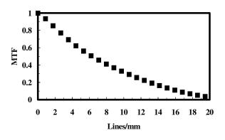
Figure 4. Modulation transfer function for the system optics
