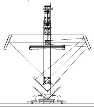
Figure 2. Bookscanner optical/mechanical design
