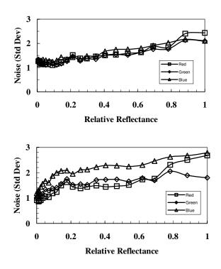
Figure 6. Temporal noise – top plot shows initial noise figure for as-captured color images while the bottom plot shows noise for color corrected images.
